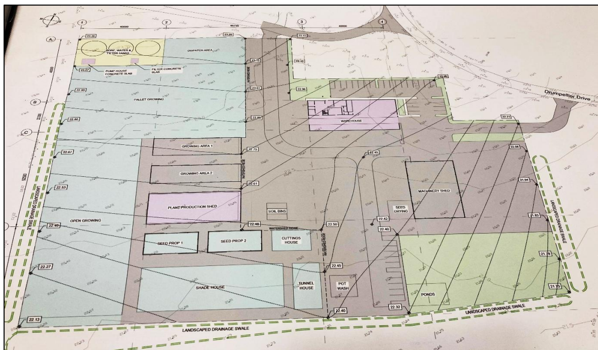
Figure 2. The new nursery plans involved bitumen hardstand around all the traffic areas to allow for heavy vehicles and deep compressed bluemetel for the growing areas. The buildings were spaced to allow machinery and trailers with adequate room to allow access by vehicles and forklifts.
