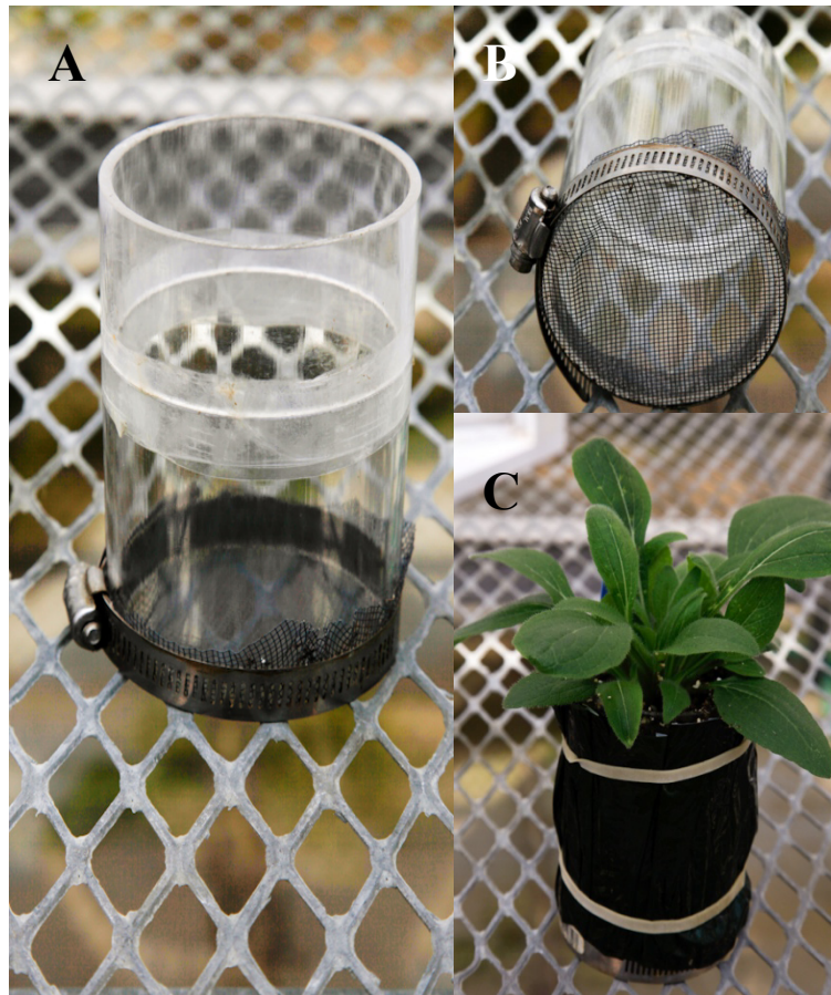
Fig. 2. (A) Design of Rhizometer illustrating the clear sided plexiglass allowing for root observations and measurements, (B) the screened bottom, and (C) a complete planted Rhizometer.
