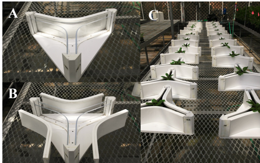
Fig. 1. (A) Design of the mini Horhizotron illustrating the three quadrant configuration, (B) removable shade panels, and (C) use in plant growth study.
