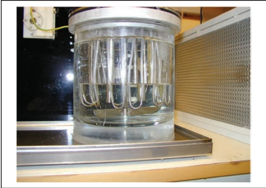
Figure 2. One of the bioreactors constructed and built at the Norwegian University of Life Sciences showing the loosely hanging silicone tubing and the pitch-blade propeller inside the bioreactor. The double jacket container to provide temperature control is also visible. The reactor has just come out of the autoclave where it has been sterilised together with one litre liquid medium. It has been calibrated and is now ready for inoculation of cells.
