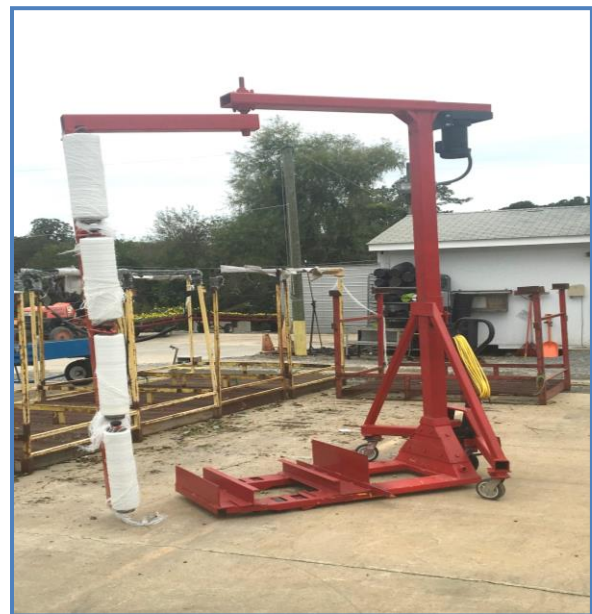
Figure 3. On-site, nursery-built machine for wrapping pallets with plastic to prevent plants from moving and falling during shipping.
