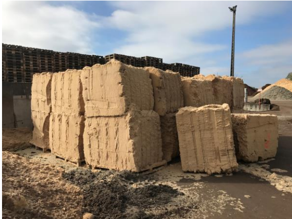
Figure 3. Some wood fiber materials can be easily compressed in different sized bales to aid in storage and transport.
