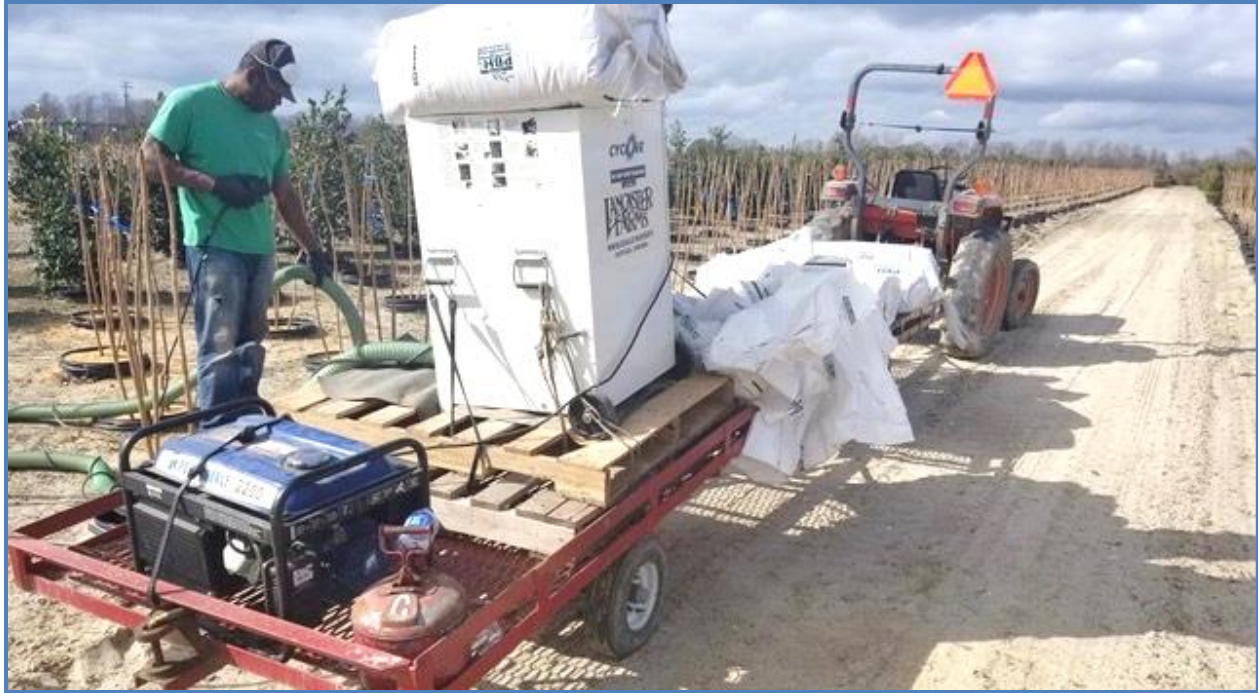
Figure 2. Using an insulation blower to apply rice hulls as a weed barrier to the tops of containers.
