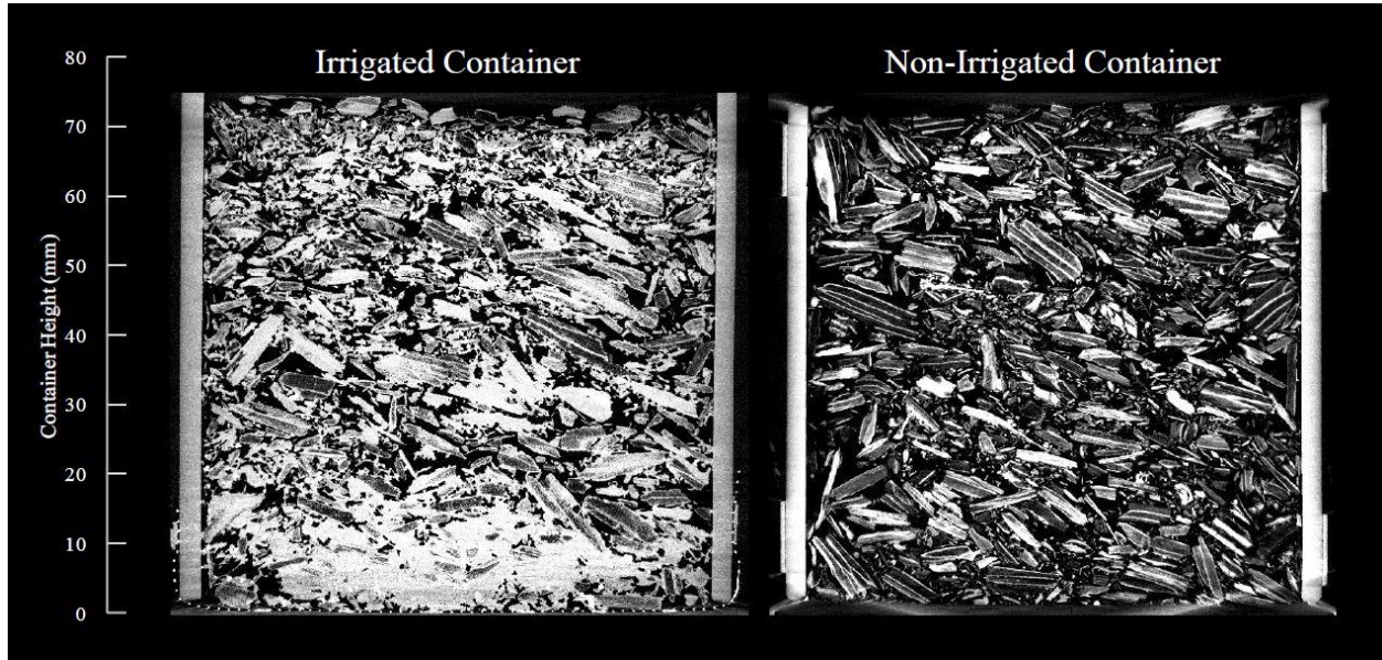
Figure 5. Pine bark cores were analyzed before and after irrigation. White or light grey objects indicate the presence of solids and water. Black spaces indicate air-filled regions.
