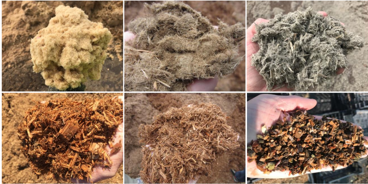
Figure 1. Wood substrate materials from European and North American manufacturers show variations in particle size and structure.
