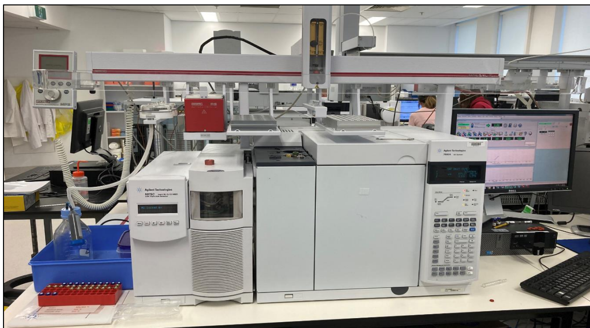
Figure 2. Single quadrupole GC/MSD instrument (Agilent Technologies, Palo Alto, CA, USA) retrofitted with a MPS 2 Gerstel Multipurpose sampler (Gerstel GmbH & Co. KG, Germany).
