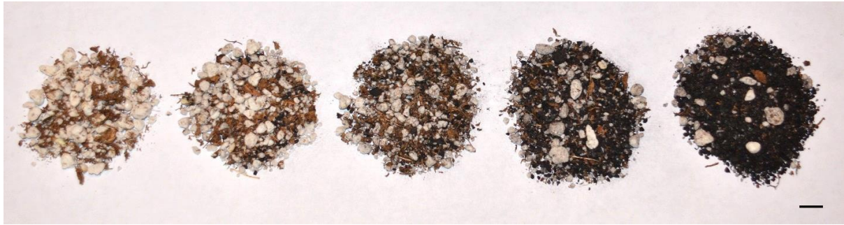
Figure 2. Sphagnum peat and coarse perlite (1:2, v/v) substrate amended with coconut-shell biochar at 0, 10, 20, 40, and 80% (left to right, v/v, bar = 1 cm).
