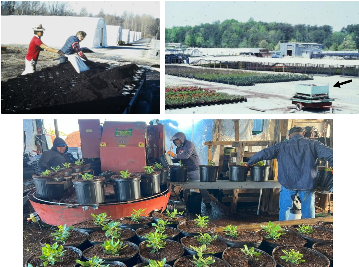
Figure 8. (top, left) container hand-filling in 1984, (top, right) a custom made portable potting machine (arrow), and (bottom) automated container potting machine used today.
